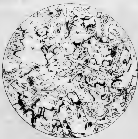
Fig 3. Petrographical from Copper River Mrs. Rich. Ordinary light shows as somewhat Opaque (1); some alteration product of argillite (2); thin brown magnetite (3); peridotite (4) and opatite (5)
