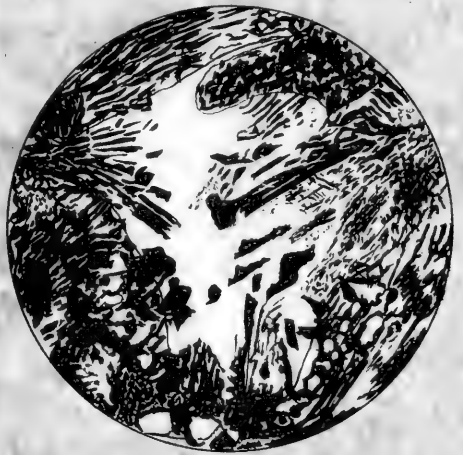
Fig. 4 from large area of red rock in the gabbro of Duluth Minn. Polarized light. Scale 25 diameters. Orthoclase decomposed and saturated with corrosion quartz, the numerous areas of which belong to only six individuals
