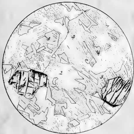
Figs 1 and 2 coarse olivine-diabase or olivine-gabbro from French River Minnesota Scale 25 diameters Fig 1 ordinary light Fig 2 polarized light See pages II, 281 Olivine (1); anorthite (2); diopsidic augite (3)
