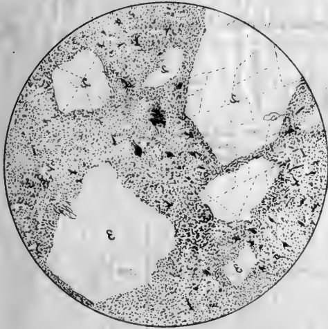
Fig. 2. Matrix of quartz-porphyr from Terek Lake horizon, Krasnodar Terr. Ordovician level. Scale is 0.5 mm. (1) - matrix; (2) - quartz; (3) - orthoclase.
