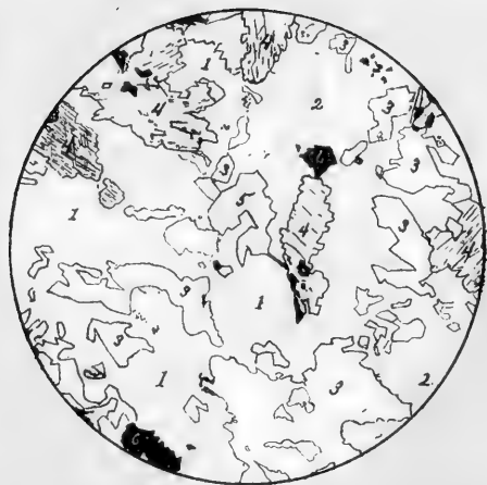
Fig. 1 Uralitic augite-syenite, Duluth, Minn. Ordinary light. Scale 20 diameters. Orthoclase (1) and oligoclase (2) saturated with secondary or corrosion quartz (3) , which sometimes forms large areas; uranite pseudomorphs (4) after augite; chlorite (5) , magnetite (6) .
