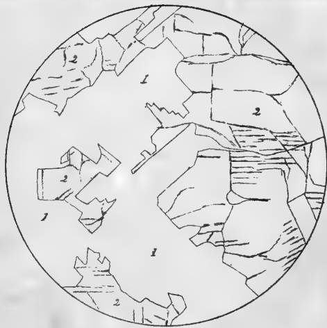
Figs. 1 and 2. Diabase or gabbro from coast of Lake Superior, near Beaver Bay, Minn. 1 Fig. 1. ordinary light. Fig. 2. polarized light. Scale 21 diameters Anorthite(1), augite(2).
