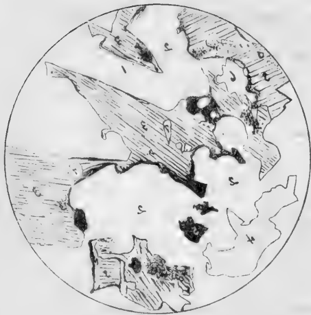
Fig. 2. Hornblende gabbro from Ashland County, Minn. Oligoclase (O); orthoclase (A); hornblende (H); quartz (Q); magnetite (M); ilmenite (I); calcite (C); apatite (P).
