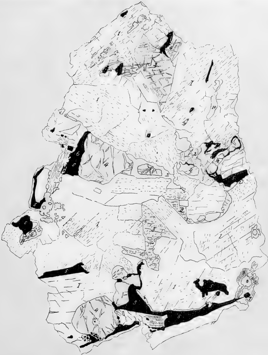
Coarse Olivine-Gabbro from Bladder Lake, Wis.; Ordinary light. Scale 10 diameters Labradorite(1); augite(2); diopside(3); olivine(4); titaniferous magnetite(5); biotite(6); Secondary zo olivine, biotite(7); iron-oxide(8); talc; viridite(10).
