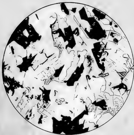
Fig. 1 Hornblende-gabbro from Ashland County, Wis. Ordinary light. Scale 35 diameters Labradorite (1); orthoclase (2); augite (3) largely altered to verdite and uvalite; brown hornblende (4); titaniferous magnetite (5); apatite (6).
