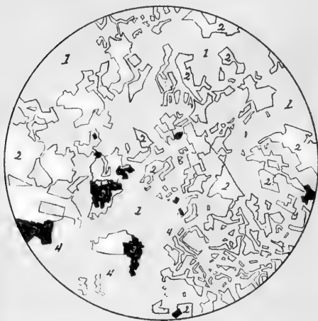
Fig. 3 Granitic porphyry from Ironton Trail, Ashland County, Wis. Ordinary light. Scale 27 diameters. Reddened feldspar, saturated with secondary quartz (1) ; magnetite (3) , greenish alteration product (4)
