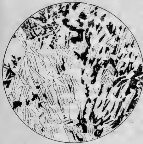
Fig 4. Petrographical from Copper River Mrs. Rich. Ordinary light. Shows as somewhat Opaque (1); some alteration product of argillite (2); thin brown magnetite (3); peridotite (4) and opatite (5)
