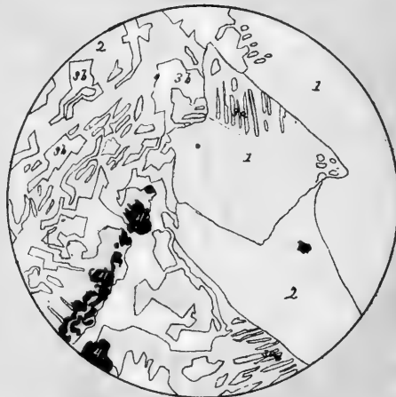
Fig. 4 Augite-syenite from pebble in conglomerate, Mt. Bohemia, Keweenaw Point, Mich. Ordinary light. Scale 27 diameters. Orthoclase (1) (trinned) and labradorite (2) both saturated with secondary quartz arranged in fine lines (3) and in regularly outlined areas (4) of augite
