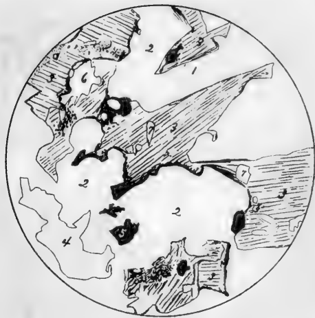
Fig. 2 Hornblende-gabbro from Ashland County, Wis. Ordinary light. Scale 35 diameters Oligoclase (1); orthoclase (2); brown hornblende (3); uvalite (4), altered from diallage; titaniferous magnetite (5); quartz (6); apatite (7).
