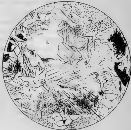
Fig. 5. Hornblende gabbro from English Lake, Minn. Oligoclase (O); orthoclase (A); quartz (Q); hornblende (H); magnetite (M); ilmenite (I); calcite (C); apatite (P).
