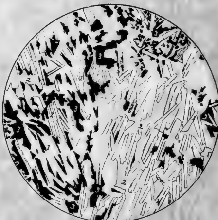
Fig. 4 Diabase from north shore of Lake Superior, near Split Rock River, Minn. Polarized light. Scale 32 diameters Labradorite (1) in small tabular crystals arranged in a common direction; augite (2) in large areas each including many plagioclases; magnetite (3) in the interspaces of the augites
