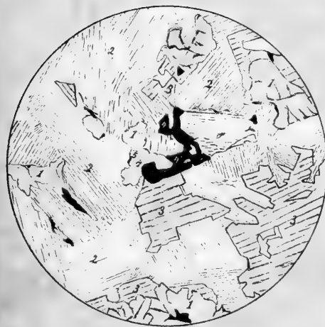
Figs 3 coarse olivine-diabase or olivine-gabbro from north shore Lake Superior, near Sucher River, Minn. Scale 25 diameters. Ordinary light. See pp 281 and 287 Olivine (1); anorthite (2); diopsidic augite (3); titaniferous magnetite (4); green alteration product of olivine (5)
