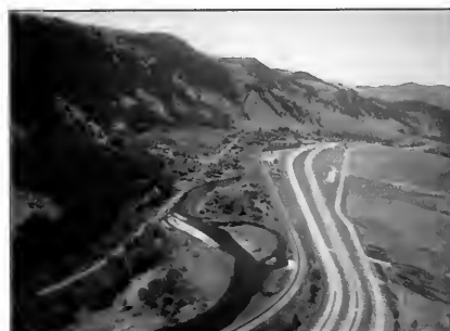
Rivers constrained by extensive highway and railroad embankments may suffer widespread instability.
