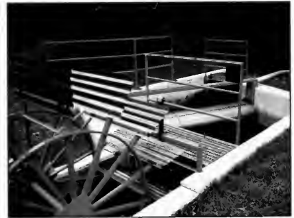
Large drum screens can accommodate a wide range of flows (from 5 to 50 cfs or more).
