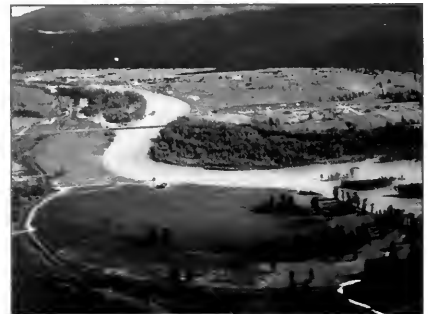
Replacement trees are colonizing the expanding point bar floodplain. The channel is moving several feet per year (20+ ft. in 1997), much to the dismay of the landowner.
