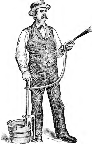
FIG. 129.—A foot pump of great efficiency. Such a pump is better operated by two persons to get the best results. (Commission of Horticulture.)
