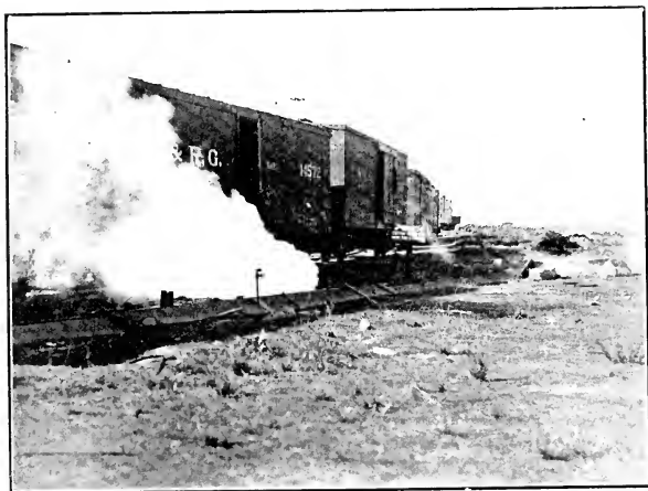
FIG. 107.—Volume of steam used for disinfecting cotton cars. (Photo by L. A. Whitney.)
