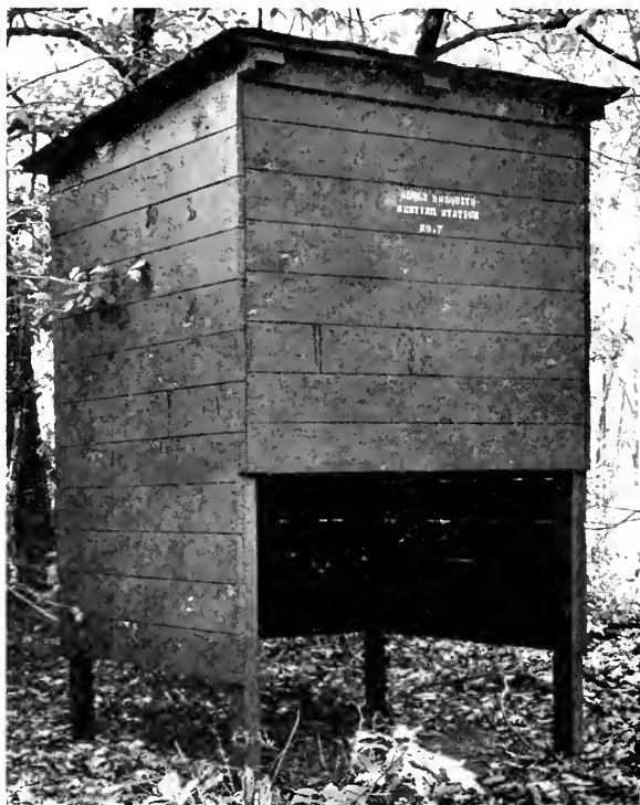
Fig. 1. Artificial shelter for measuring mosquito densities (U. S. Army Signal Corps photograph).
