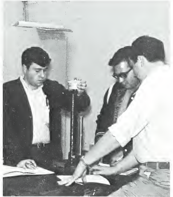
Obtaining demensions with vernier height gauge.
