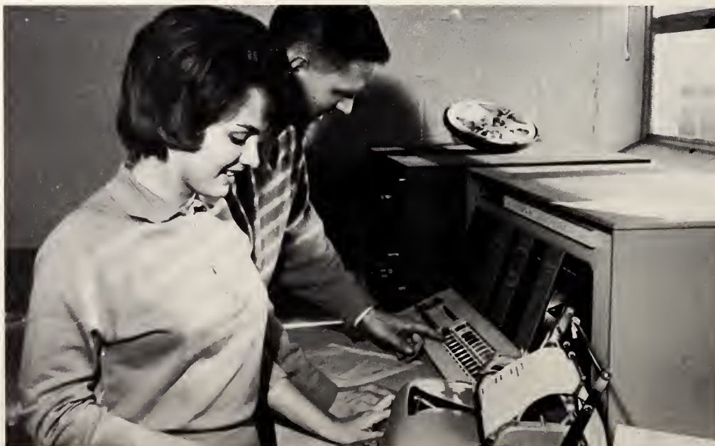
Testing panel wiring on the 407 Accounting machine.
