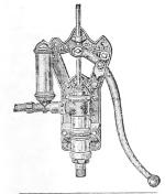
Fig. 566.—This is made of cast brass excepting frame and lever, and capable of doing better work than the cheaper Portable Force Pump. They may be used as a small House Force Pump, where large ones can not be used.
