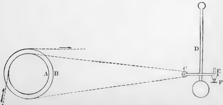
FIG. 30.—The principle of the Serigraph (original).
