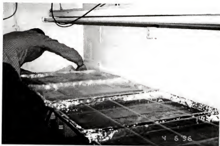
Step 5. The trays containing the mycelial homogenate are covered with clear polyethylene film.
