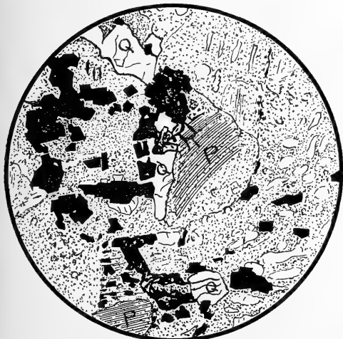
Fig. 9 Altered micaceous gneiss from the Hook district. Actual size 3 mm. Q, quartz; P, plagioclase; black, magnetite from biotite
