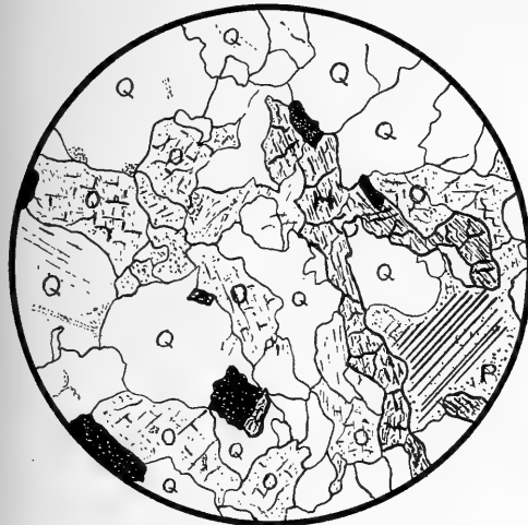
Fig. 2 Bald hill granite gneiss. Actual size 3 mm. Q, quartz; O, orthoclase; P, plagioclase; H, hornblende; black, magnetite
