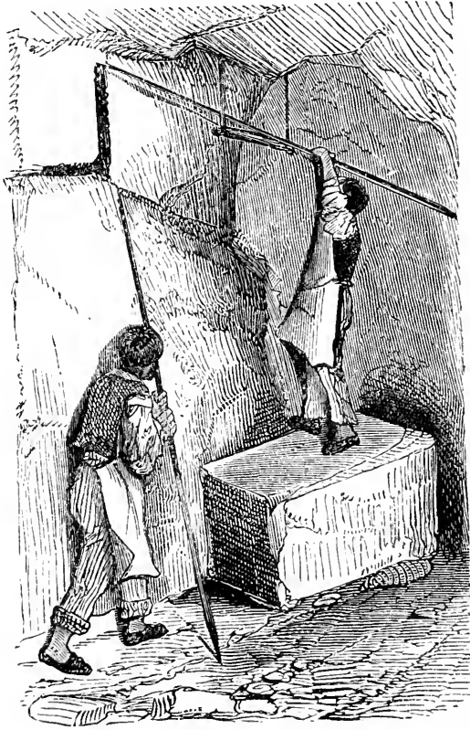
Fig. 24. Extracting the stone in subterranean quarries.
