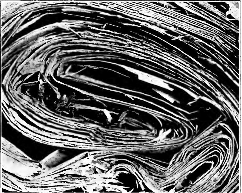
! FIG. 2. DECAY CAUSED BY FOMITIPORIA WEIRII MURRILL
