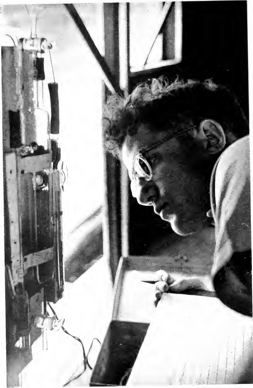
ANALYZING THE SULPHUR-DIOXIDE CONTENT OF THE AIR FROM AN AIRCRAFT.
