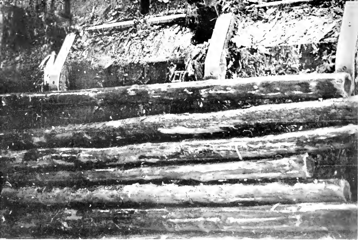
Small 16-foot logs on a sawmill log-deck. Log sizes may be gauged by comparing with the steel straps which are about five inches wide. Stumpage payable on these logs when measured by the Doyle rule will be less than four cents each. They will each yield about 30 board feet of comparatively low-grade lumber.
