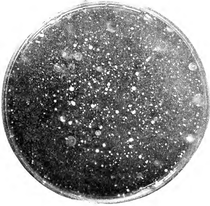
Gelatine plate exposed to the deposition of germs and moulds for one minute in a barn when some of the above operations were in progress.
