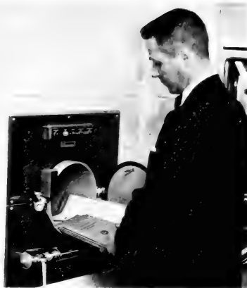
Removing "clean" pamphlets from pass-clave in outside hall after overnight treatment.
