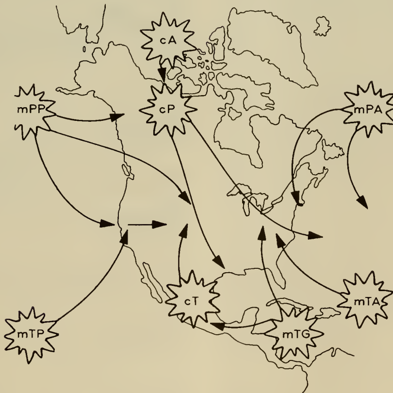
Figure 2.7 Air masses: cA , Continental Arctic; cP Continental Polar, a source of very cold winters; mPP , Maritime Polar Pacific, a source of cool moist winds; mTP , Maritime Tropical Pacific, a winter source of warm moist winds; cT , Continental Tropical, a source of dry hot winds; mTG , Maritime Tropical Gulf, a source of warm moist winds; mTA , Maritime Tropical Atlantic, a source of warm moist winds; mPA , Maritime Polar Atlantic, a source of cool moist winds.
