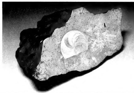
Above: Test grinding of the Santa Rosa meteorite left a nearly circular hole 46 millimeters across and less than a millimeter deep. Below: Artist's conception of the Mars rover Opportunity, sampling an iron meteorite on the Martian surface.
