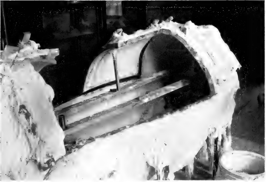
A portion of the piece mold with clay model removed. This has on its interior, of course, a perfect impression of the hippo model, and will give a positive or cast of this impression to soft plaster placed against this interior. The mold of the hippo was thirteen feet long
