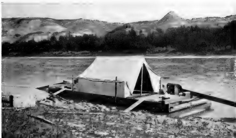
Flatboat constructed for drifting down Red Deer River. A twenty-two-foot sweep at each end, like a long oar, served in guiding the boat out of the way of rocks in the course. This was eventually converted into a houseboat because of excessive rains and dearth of camping places along the shores
