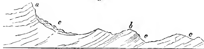
a. Pentamerus limestone. e. Talus. b. Thin-bedded waterlimes. c, c. Hudson-river series.
