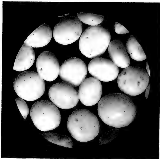
No. 3.—Top bed, Liverton Ironstone. Oolitic grains; insoluble portion left on boiling with strong Hydrochloric acid. Magnified 30 diameters.
