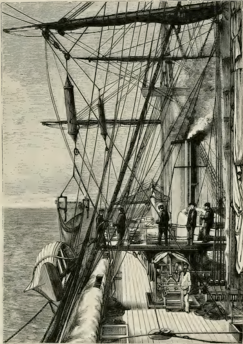
DREDGING AND SOUNDING ARRANGEMENTS ON BOARD THE "CHALLENGER."
