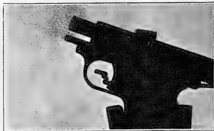
FIG. 2.—Automatic pistol; empty cartridge case just emerging from the receiver.
