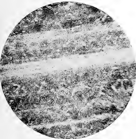
FIG. 3.—Mild steel (with 0.7 per cent. manganese). Longitudinal section \times 100 (treated 900° water : 700° water).
