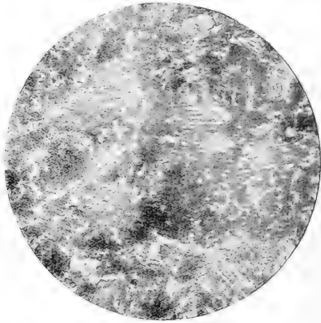
FIG. 4.—Mild Steel (with 0.7 per cent. manganese). Transverse section \times 600 (treated 900° water : 700° water).
