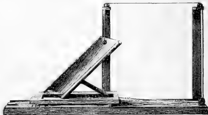
FIG. 35.—Model to illustrate the aberration of light. A square tube, with glass front and a slit along the centre of its upper side to allow the passage of a thread, is inclined at 45° and caused to run along a level track, while a weight suspended from a thread passing round three pulleys and attached at the other end to the front of the carriage is allowed to descend. In this figure the weight is at the commencement of its fall.
