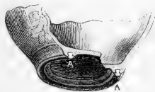
FIG. 2.—Arrangement of the india-rubber covering in a swallow-tail groove AA, provided at the base of the object.
