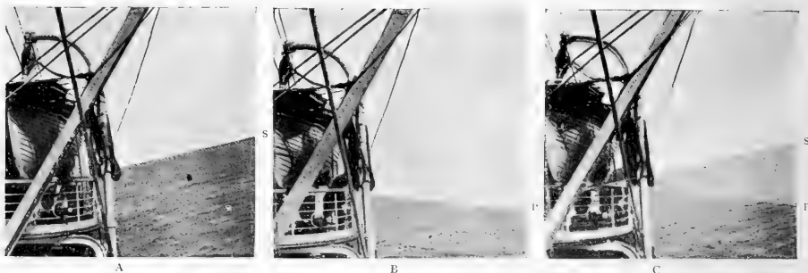
Union Steamship Co.'s Mokoia . Rolling angle found by photography. A is a picture taken at the instant of the end of rolling to the right, s; B is a picture taken at the instant of the end of rolling to the left, r; C is a composite picture made by superposing the two films, A and B. The pictures of the ship are made to coincide, thus the angle between the two horizons in A and B is found. Lat. 34° 27' S. Long. 157° 45' E. To Sydney 325 miles.
