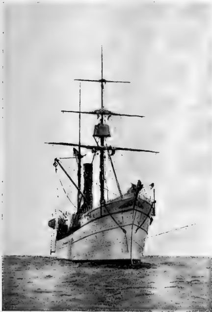
The U.S. steamer Albatross dredging, showing port boom rigged for surface towing.
