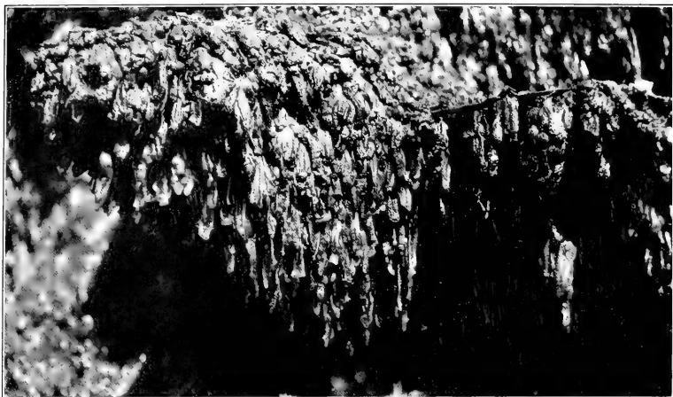
FIG. 18.—Type and amount of fouling on ships' bottoms. Large clusters of tunicates (sea squirts)
