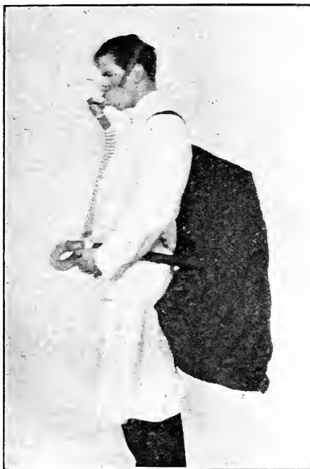
FIG. 2.—Bag, pipe, tap, valves, and mouthpiece used to investigate the gaseous exchanges of man during running.
