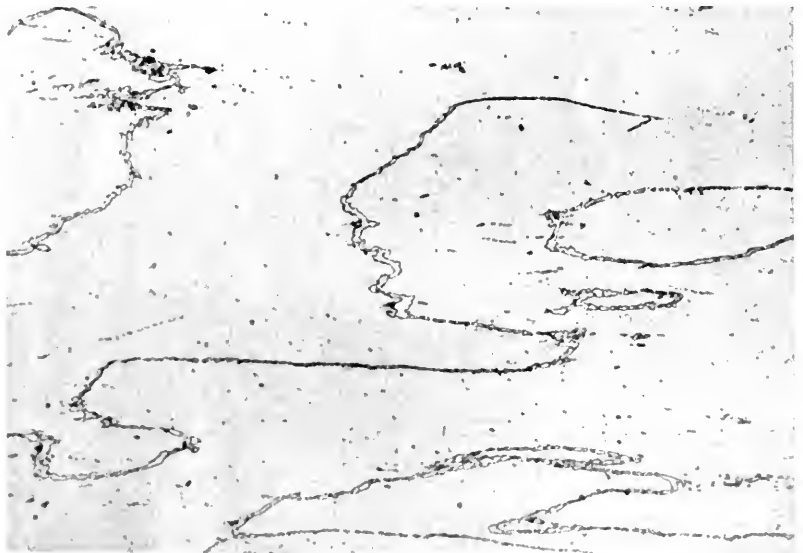
FIG. 3.—Beaded cementite at crystal boundaries of ferrite. \times 250 .
