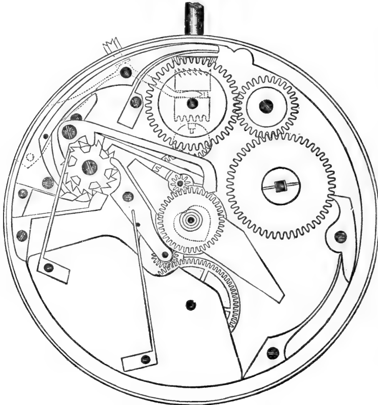
FIG. 8.—Chronograph with Swiss Keyless work.
