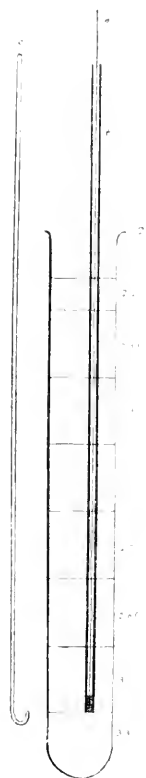
A test-tube containing a diffusion column. The figures at the side indicate corresponding specific gravities: A, pipette fitted with a piston; B, crook by which the lower end of the pipette may be plugged.
