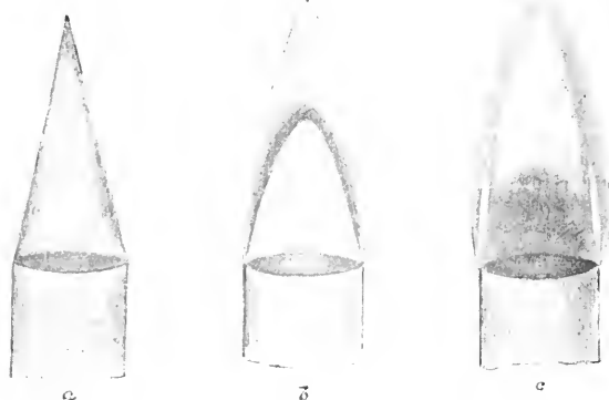
FIG. 2.—Typical Flames. (a) Carbon monoxide, single coned; (b) Cyanogen, two coned; (c) Small coal-gas flame.
