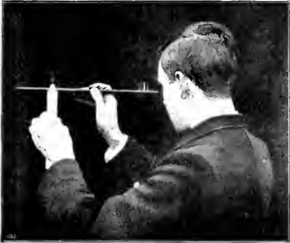
FIG. 1.—A simple form of spectroscope.
