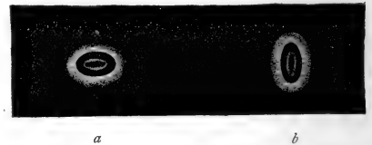
FIG. 5.—Elliptic rings produced by astigmatism.
