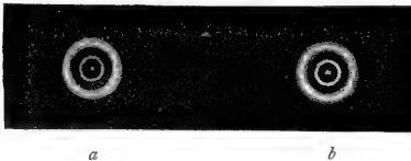
FIG. 3.—Appearances due to spherical aberration.
