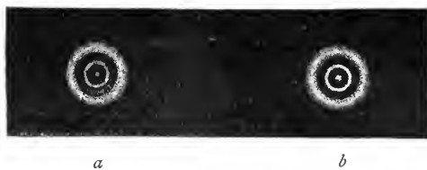
FIG. 3.—Appearances due to spherical aberration.
