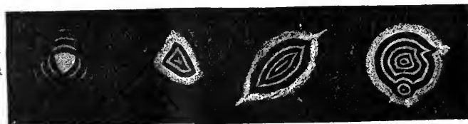
FIG. 6.—Diagrams showing effects due to (a) flexure; (b and c) strain in cell; (d) veins in objective.
