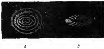
FIG. 2.—Appearances observed when the objective is out of square.
