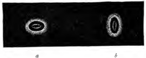
FIG. 5.—Elliptic rings produced by astigmatism.
