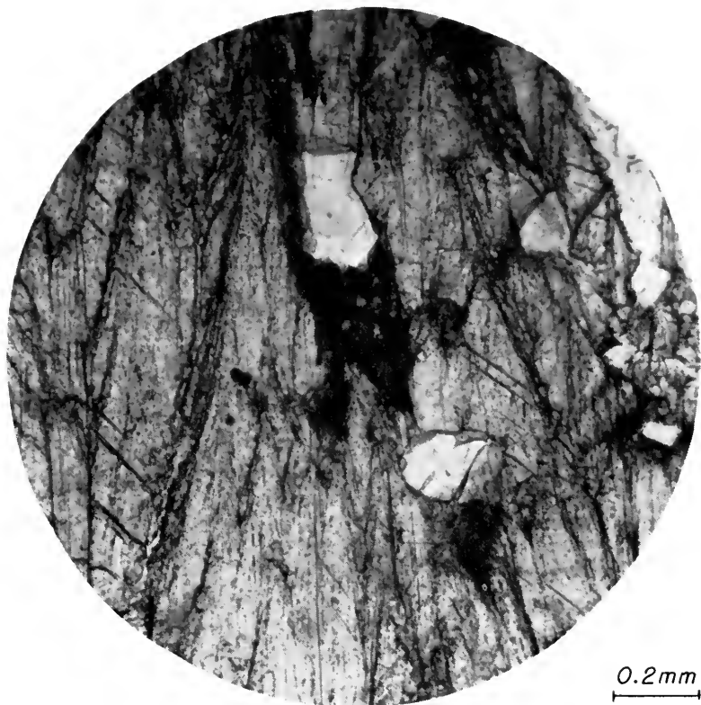
FIG. 83. Vertical thin section of coned calcite veins in sandstone showing quartz grains and associated clay "caps." Near Greybull, Wyoming (slide no. 284)
