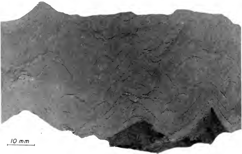
FIG. 38. Polished vertical section of cone-in-cone layer showing corrugated cone cups in lower center and right. Dotson's Branch, Parke County, Indiana (G-3554).
