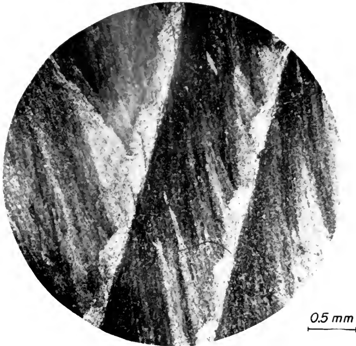
FIG. 54. Vertical thin section of cone-in-cone layer showing corrugated clay layers and calcite spindles; crossed nicols. North East, Pennsylvania (slide no. 276).
