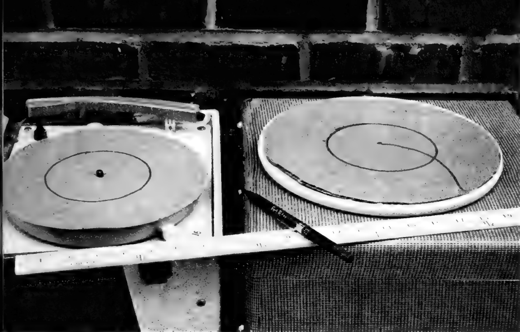
This photo shows cardboard disks mounted on a record-player turntable (left) and on a plastic "lazy Susan" turntable (on box at right). How were the circles drawn without moving the felt tip of the marking pen?
