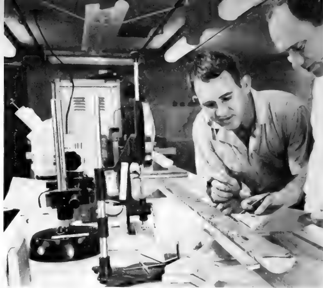
Scientists study a split core of sea-floor sediment in the Core Laboratory aboard the Glomar Challenger . Cores are examined and photographed before being stored in a refrigerator for dating and further study ashore.
