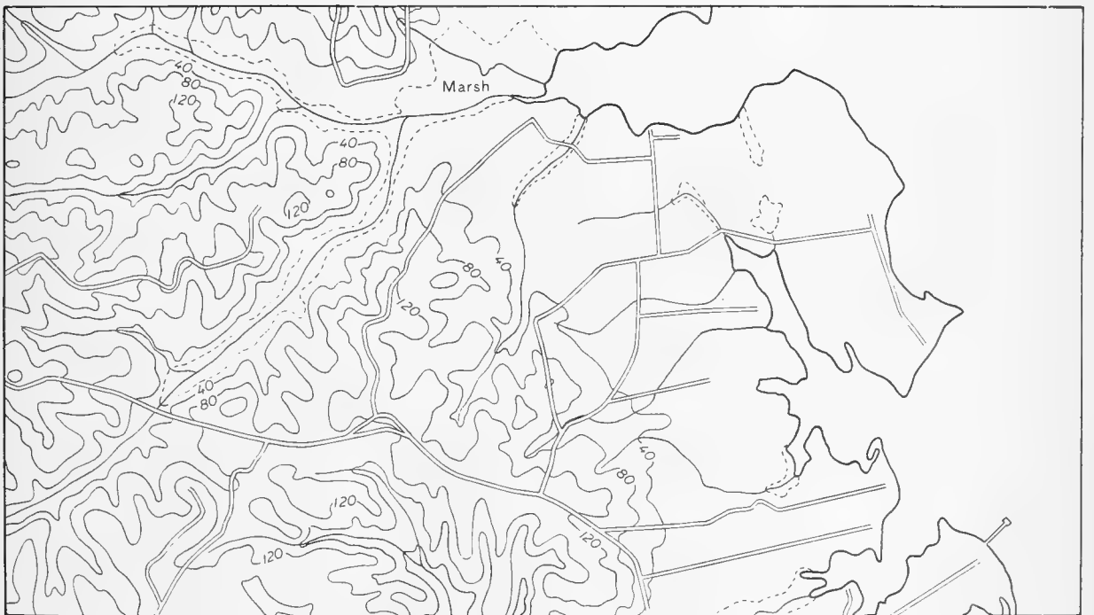
Nautical chart compilation showing generalization of contours taken from Geological Survey quadrangle map shown above.
