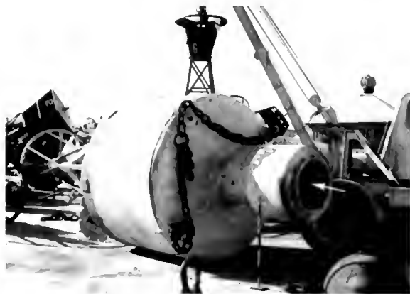
FIG. 1. Typical navigation buoy. Arrow indicates the sheltered, inner portion of the stabilizer tube.
