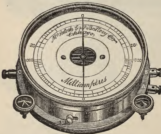
Fig. 12. McIntosh Milliampère Meter. b (Fig. 12), for stronger currents at c and a .
