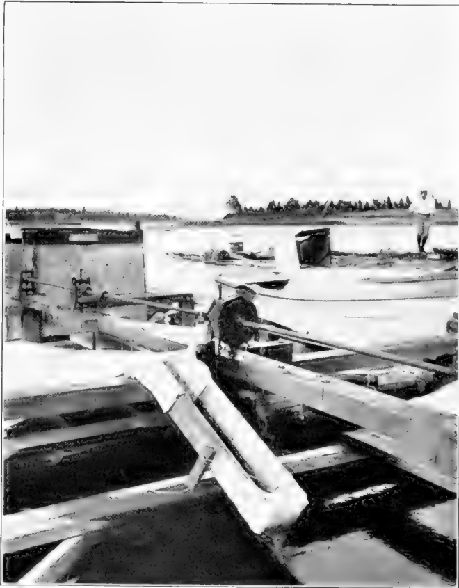
FIG. 15.—Filter car, same as figure 14, plate xcvr, showing bucket chain in operation. One of the buckets has just emptied itself and the stream of water is faintly shown running into the trough.
