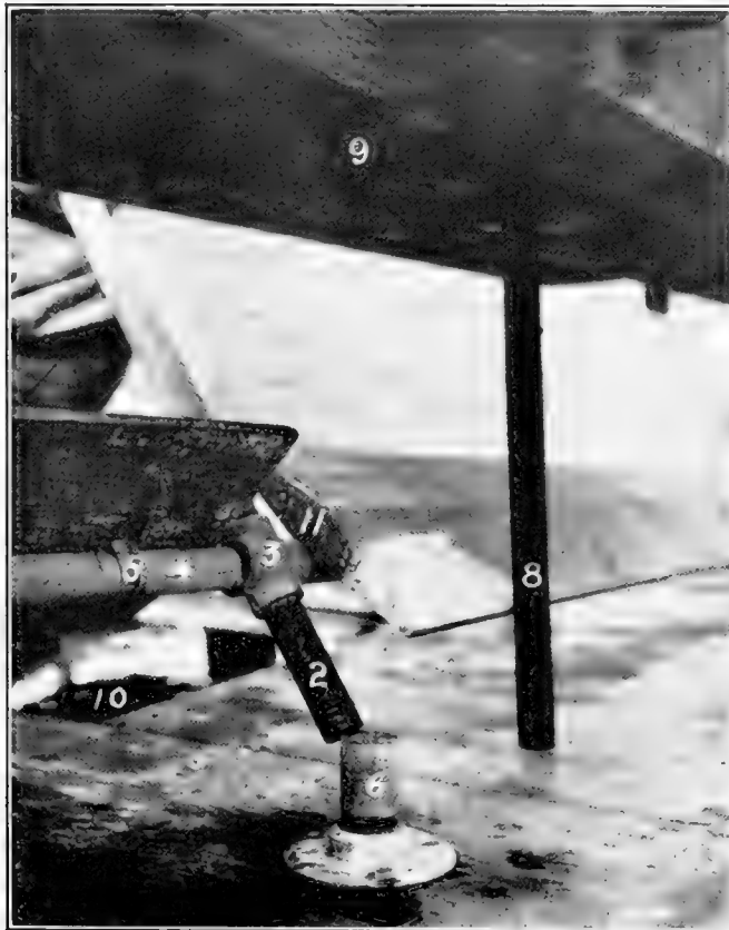
FIG. 18.—Detail of lower portion of the propeller shaft and its socket in floor of car. 1, propeller shaft, made of gas pipe; 2, short portion of shaft made of steel, to fit into the socket (6); 3, four-way pipe coupling; 4, gas pipe to which blades are strapped; 5, strap holding propeller blades; 6 and 7, socket and flange; 8, upper disconnected steel portion of the propeller shaft; 9, shaft beam; 10, window in bottom of car; 11, base of propeller blade, showing in section the shape.
