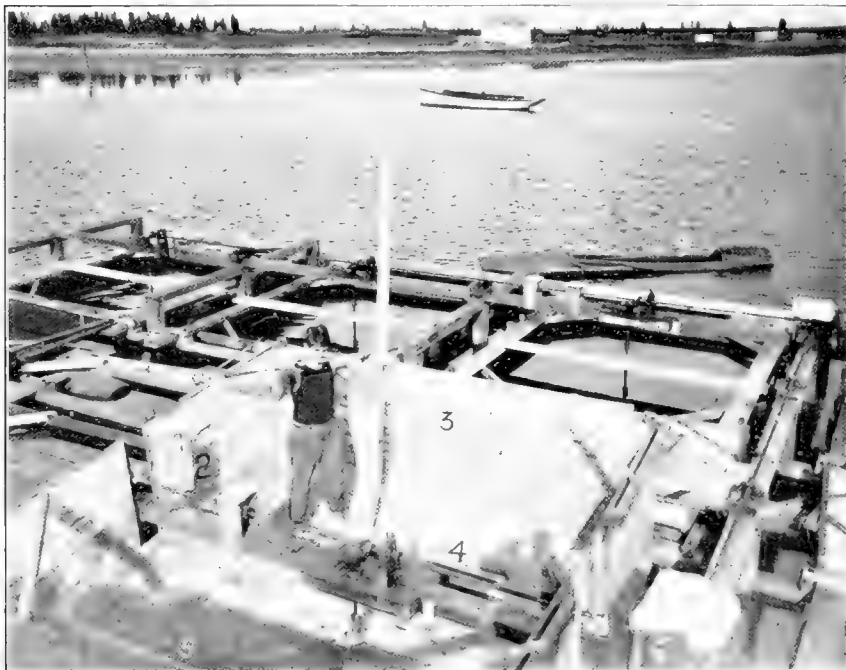
FIG. 6.—Interior of rearing car, and propeller. 1, slot in end of car; 2, doors for closing the slot; 3, side screen windows; 4 and 5, bottom windows; 6, box covering gear trains; 7, transverse shaft; 8, longitudinal shaft; 9, towing car. The arrangement of shafting on farther float can be seen.
