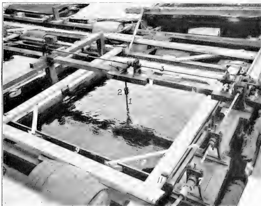
FIG. 4.—Car with propeller in motion. From propeller the shafting may be followed back (1-5) to the universal joint. 1, propeller shaft; 2, sleeve coupling; 3, longitudinal shaft; 4, adjustable shaft hanger; 5, gear trains from longitudinal to transverse shafts; 6, transverse horizontal shaft of float; 7, shaft hanger; 8, ball joint connecting shaft with that of house boat; 9, edge of rearing box; 10, brace across corner of rearing box; 11, holding-down plank mortised into corner post; 12, shaft beam.
