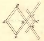
compass-joints; at B is a point, which serves to fix the instrument to the drawing board; at A is a point which is made to pass round the figure to be reduced or enlarged; at C is a hole for a pencil pressed down by a weight, and the pencil traces the similar figure, altered in dimensions in the ratio of BC: AB or BF: AD.
