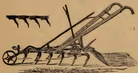
FIG. 40. THE "PLANET JR." TWELVE TOOTH HARROW, CULTIVATOR AND PULVERIZER. PRICE, PLAIN, $8.50. WITH WHEEL, COMPLETE, PRICE, $12.
