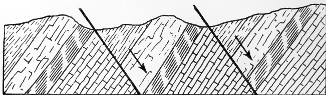
Fig. 2 Normal faulting in inclined strata; the same beds outcrop repeatedly when traced across the strike
