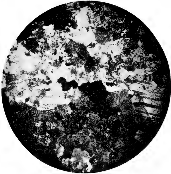
Photomicrograph of gabbro, Port Henry. Constituents are pyroxene, feldspar and magnetite.
