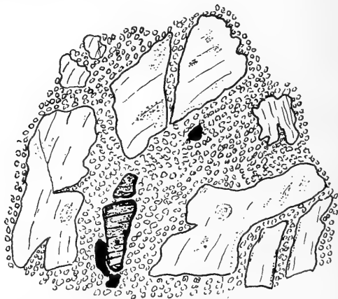
Fig. 8. Microscopic appearance of syenite from near Harrisville. Shows groundmass of crushed feldspar, with larger fragments of the original crystals, also a little pyroxene and magnetite
