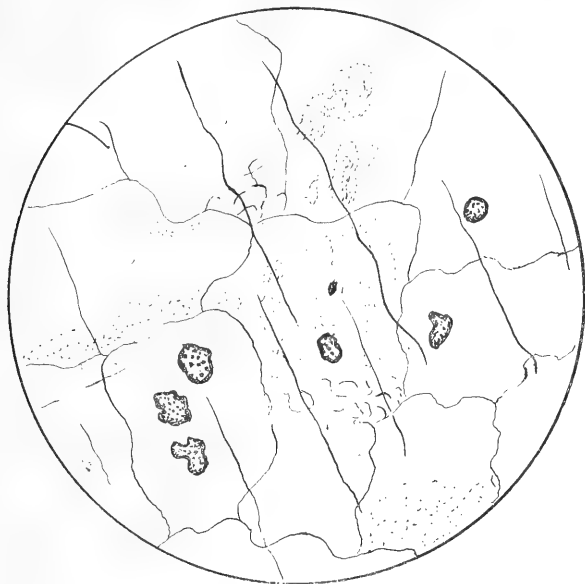
Fig. 5 Microscopic fractures in anorthosite, parallel to the rift or direction of easiest cleavage. The section is nearly pure feldspar, the small grains being garnet. Enlarged 25 times
