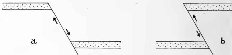
Fig. 1 Simple faults. a illustrates the common or normal fault, and b the reversed fault
