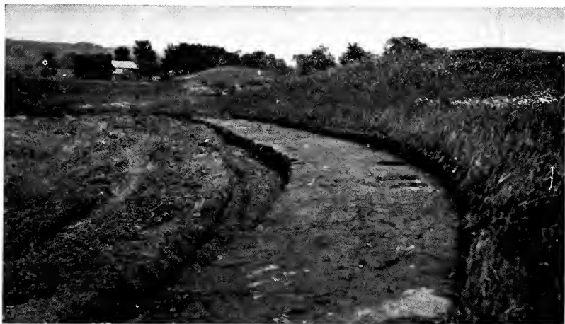
Figure 38 A typical layer of weathered molding sand so common to the Hudson river valley. The stripping and loading is all done by hand. This weathered layer tends to follow the topography.
