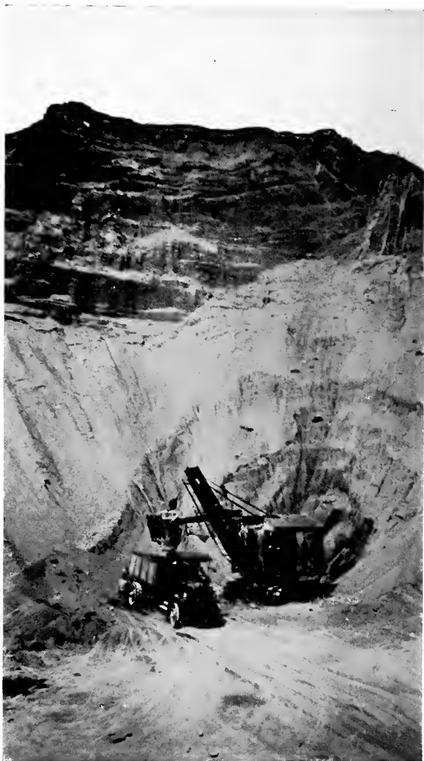
Figure 18 Power shovel loading a truck which serves as the conveyor to the plant
