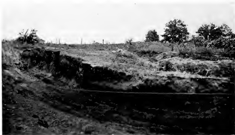
Figure 37 A river deposit of molding sand that does not owe its value to weathering
