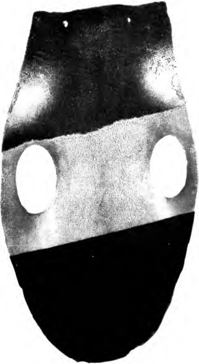
PLATE 97.—Demonstration pelt showing three stages of processing (from top to bottom) : “tanned in the hair,” with all fibers intact; “unhaired,” with guard hairs removed; and “finished,” with fur fibers straightened and dyed brown. Specimen courtesy Fonke Fur Co. (2718)
