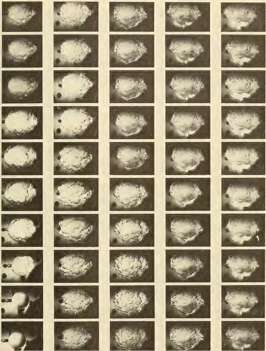
Figure 25. Sequence of bubble development from a 2-inch OD sphere. Duration of this phase, approximately 100 \mu sec.
