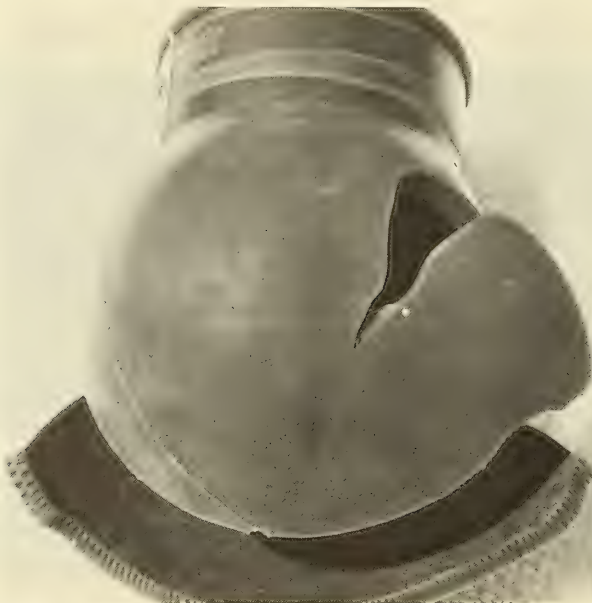
Figure 32. Close-up view of 3-inch OD rubber sphere with 0.25-inch wall after rupture.
