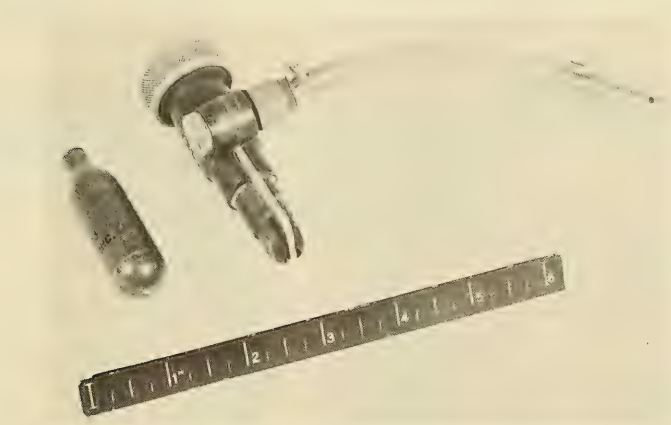
Figure 22. Pneumatic high-power/lf sound source, with 6-8 gram CO 2 cartridge.
