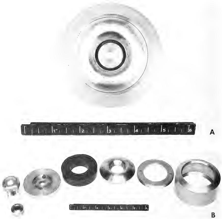
Figure 16. Experimental magnetic spark gap, (A) assembled and (B) disassembled.
