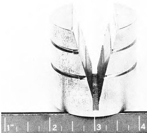
Figure 1. Basic design of horn gap (before encapsulating).
