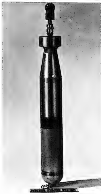
Figure 36. Acoustic bomb using Mark 15 Mod 0 pressure mechanism.
