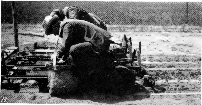
FIGURE 25.—A, Front view of sled type of seeding machine. The seed is fed by hand into the long horizontal seed trough. B, Side view of sled type of seeding machine.
