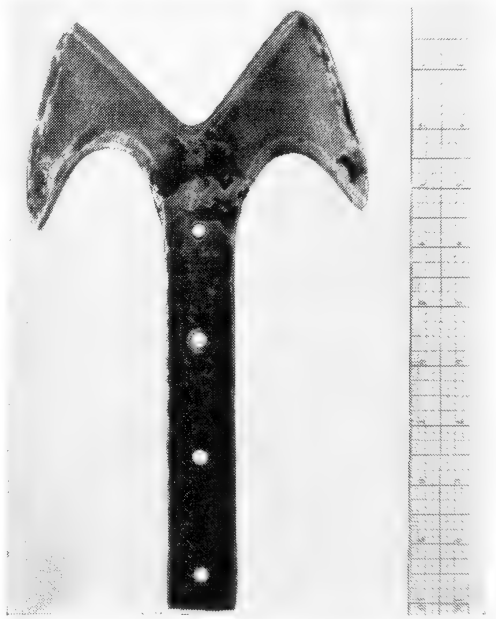
FIGURE 4.—A double-hook detacher for cutting fruit, cones, or small limbs from trees. Made from two discarded mower blades welded to a flat piece of steel 8½ inches long.
