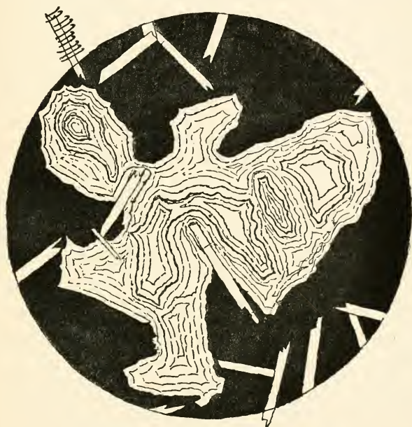
MAGMA-LAKELET, .25 mm. in size, magnified 290 diameters, from a basalt at Navingiri. The groundmass, which is a smoky devitrified glass containing abundant felspar-lathes, is coloured black. The magma-lakelet is pale yellow in the slide and displays concentric lines of congelation. It behaves like palagonite.
