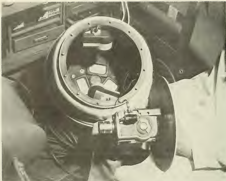
FIGURE 6 SUBSURFACE FLOAT OPENED TO SHOW CAMERA, ELECTRONIC FLASH UNITS, AND READOUT DIALS
