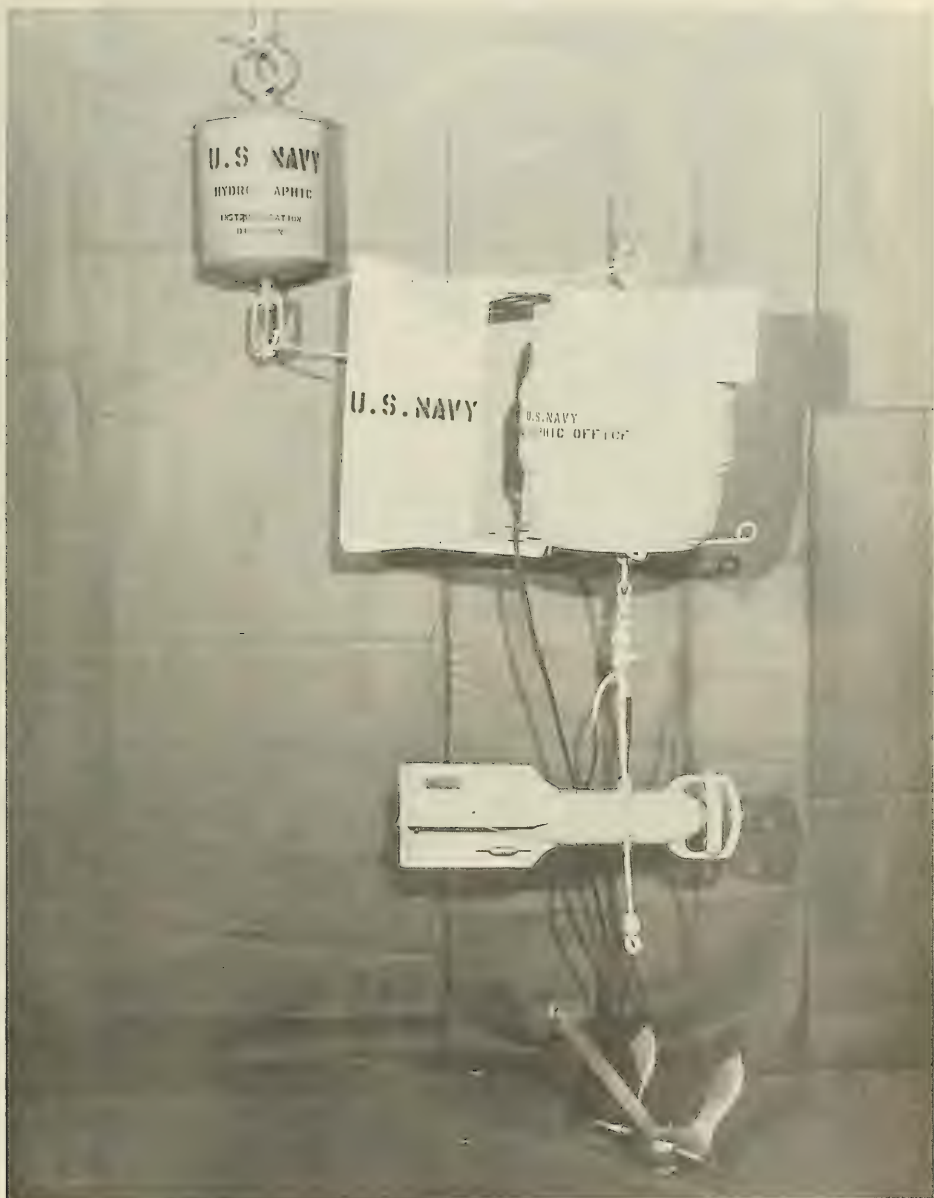
FIGURE 5 BUOYED JAPANESE CURRENT METER SYSTEM
