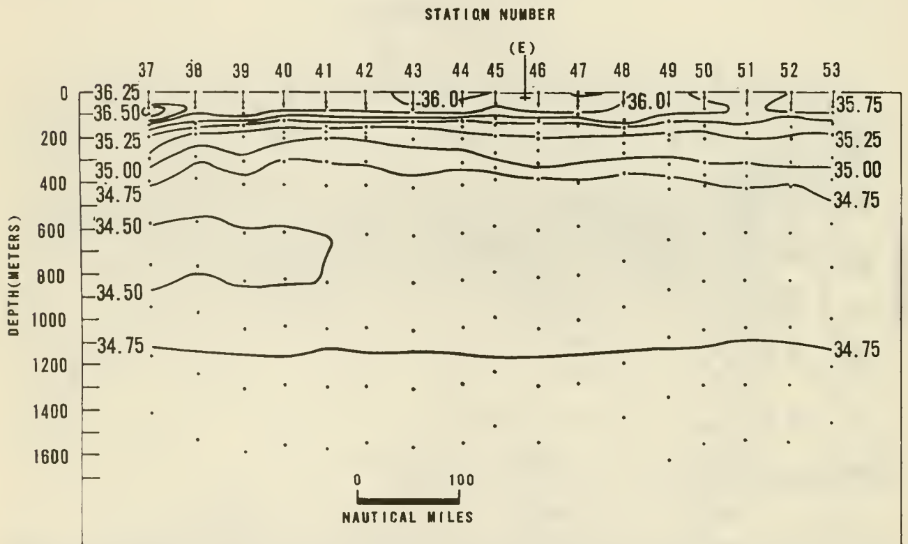
FIGURE 9. Vertical distribution of temperature ( ^{\circ}\text{C} ) and salinity ( \text{‰} ) in the upper 1700 m. Contour intervals 1^{\circ}\text{C} (except in thermocline—shaded area) and 0.25\text{‰} . Stations 37–53, 11–14 February 1966, EVERGREEN 31–779. E indicates position of equator.
